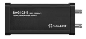
The oscilloscope can control the SAG1021I isolated USB Function/Arbitrary waveform generator to output waveform with up to 25 MHz frequency and  $\pm 3$  V amplitude. Six basic waveforms plus multiple types of arbitrary waveforms are built-in
