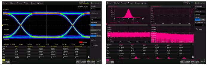
Supports eye diagram and jitter analysis/measurement. It can automatically extract the embedded reference clock from serial data and create the eye diagram. Measurement on multiple eye/jitter parameters is provided. Mask test on eye diagrams is supported
