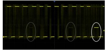
With a waveform update rate of up to 170,000 wfm/s, the oscilloscope can easily capture unusual or low-probability events. In Sequence mode, the waveform capture rate can reach 750,000 wfm/s
